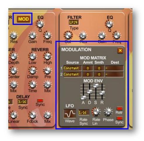
The modulation matrix is hidden under the MOD button. Press the MOD button to show the modulation matrix. Each oscillator has its own modulation matrix.
