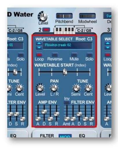
The most common sound shaping tools are available in the Mixfood Ambient Synths. Per oscillator volume level, panning, semitune and finetune, amp envelope and filter envelope. The filter itself is located in the effects section.
