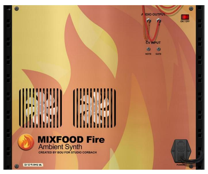
On the backside you'll find the standard stereo outputs and the standard note CV input and gate CV input.
